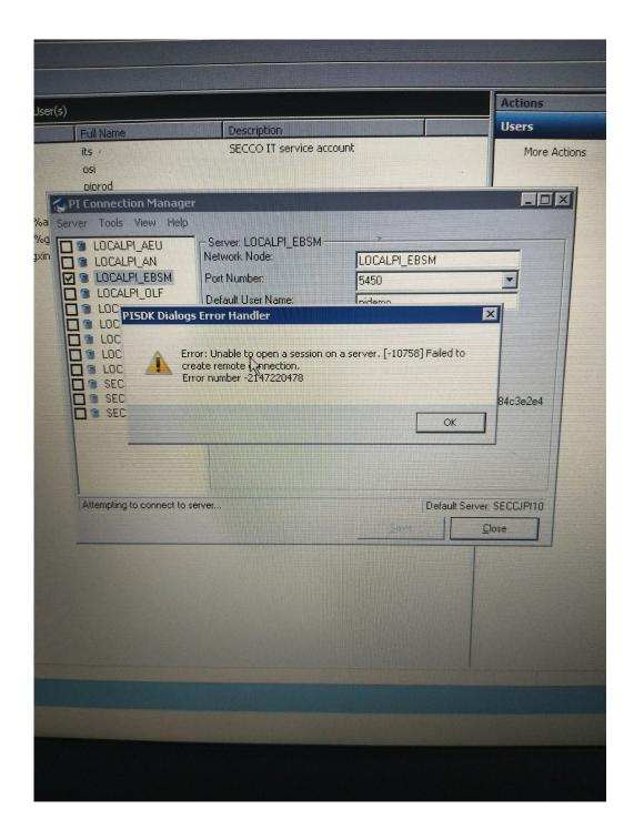
此问题为网络端至PI系统端防火墙设置,即5450端口未开放导致 https://pisquare.osisoft.com/thread/37231-error-number-2147220478
